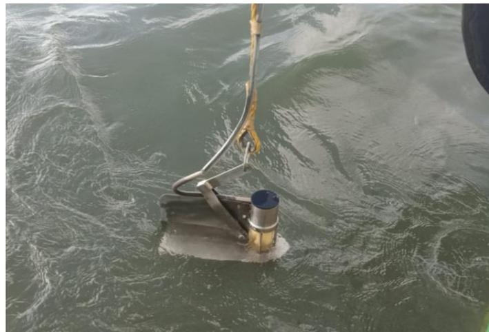
Figure 5: Ocean current meter for *in situ* measurements
