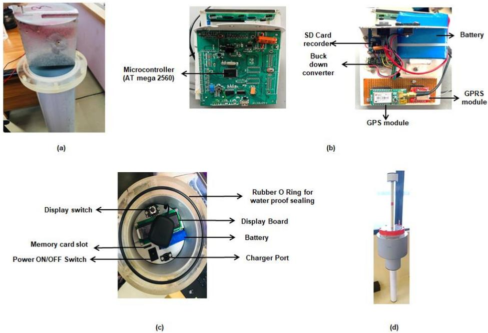
Figure 1: Assembling of drifter system components
