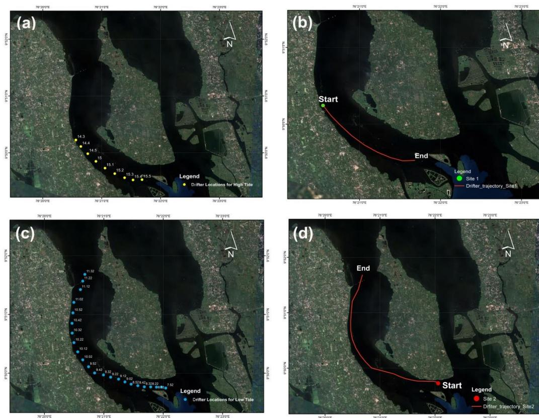
Figure 4: (a) Drifter locations during flood (high) tide phase (b) Drifter Trajectory during flood tide phase (c) Drifter locations during ebb (low) tide phase (d) Drifter Trajectory during ebb tide phase
